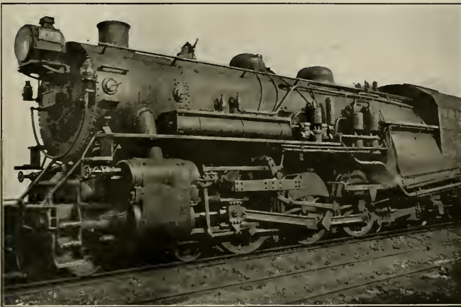
APPARATUS PLACED UNDER SMOKE BOX USED BY THE LOCOMOTIVE FEED WATER HEATER COMPANY.
